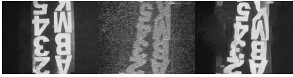
[Fig. 1] Optical image, sonar image, and style-transferred sonar image
