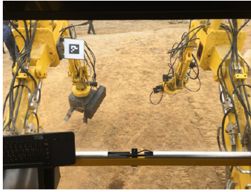
[Fig. 2] The dual hydraulic manipulators cover almost 40% of the front view of the operator, and only 60% information from the front view is provided to the operator
