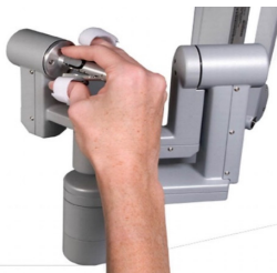
[Fig. 2] Master controller for da Vinci surgical robot
