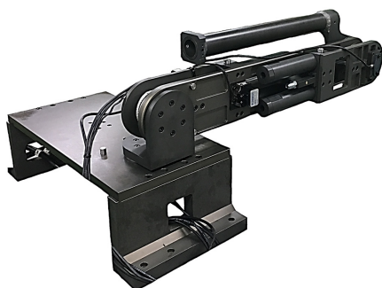
[Fig. 1] The proposed 3 DoF manipulator with cable-hydraulic actuation modules for cooperative robots
