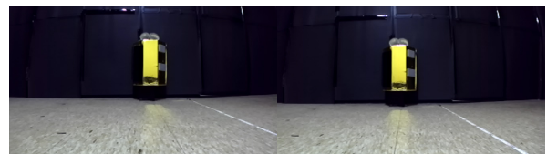
[Fig. 10] Input stereo image (Case of the distance between object and camera is 100 cm)
