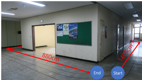
[Fig. 8] Experiment environment for IMU sensor (Rectangle corridor : 1408 x 880 cm 2 )
