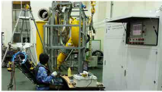
Fig. 13. Test environment of pipe cleaning robot with robot, control station and ASU
