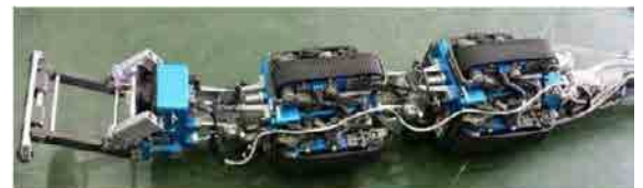
(b) Pipe cleaning robot with vacuum suction system
