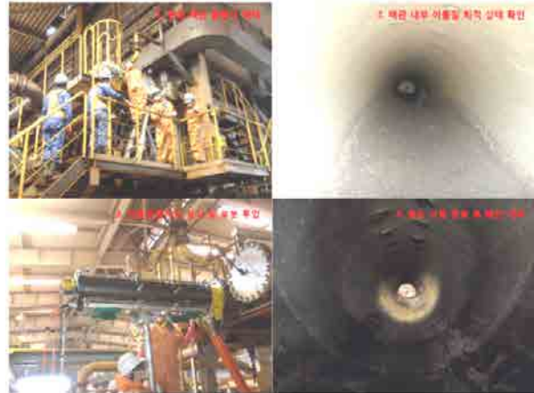
Fig. 26. Field test of the PCR using scraper moving system
