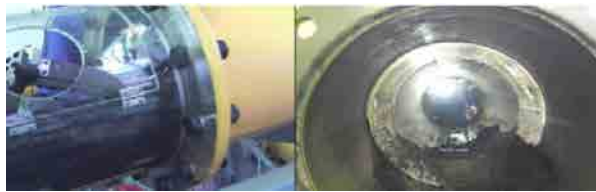
Fig. 25. Cleaning test of pipe cleaning robot with scraper moving system
