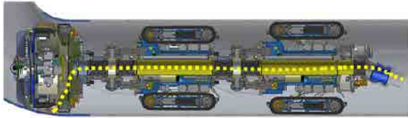
Fig. 6. Section view of pipe cleaning robot system
