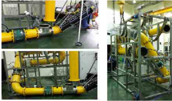
Fig. 21. Test platform of pipe cleaning robot system
