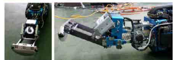
(c) Pipe cleaning robot with scraping unit system
