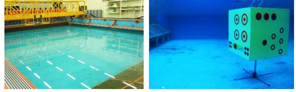
Fig. 4. KAIST test tank (left) and model scaled underwater well-head (right)
