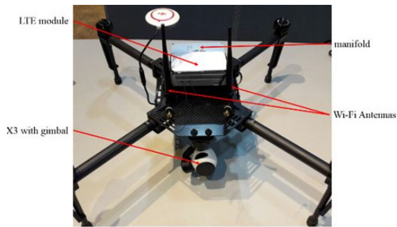
Fig. 8. The components of UAV platform
