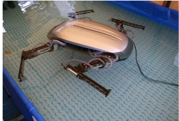
Fig. 1. Biomimetic underwater articulated robot: CALEB 10
