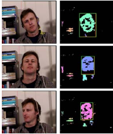
Fig. 6. Comparative results of face detection experiments: (Left) Failure of Viola-Jones method, (Right) Success of the proposed method
