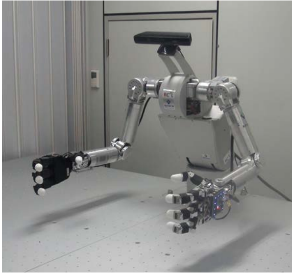
Fig. 2. KITECH's humanoid upper body system
