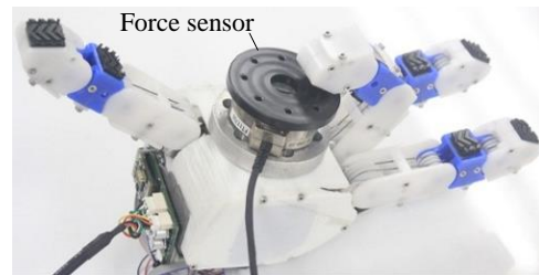
Fig. 9. Experimental setup for fingertip force measurement.
