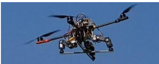
[Fig. 15] Leveling bottom of landing system during flight
