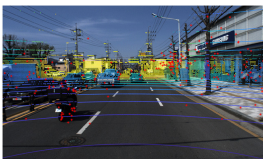
[Fig. 7] Projection of point clouds onto RGB image (example in snowy condition): colored points represents the distance and red star points are gathered from radar
