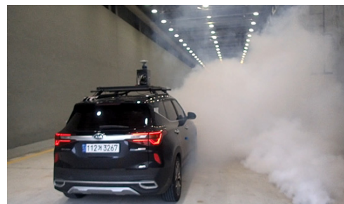
[Fig. 1] Data acquisition in adverse condition (examples of snowy and smoky conditions)
