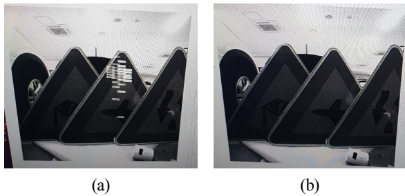
[Fig. 5] Near IR image according to trigger timing: (a) 0° trigger timing, (b) 45° trigger timing, When lidar shots forward, the return of laser affects on near IR image
