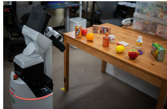
[Fig. 12] Test setup using HSR home service robot
