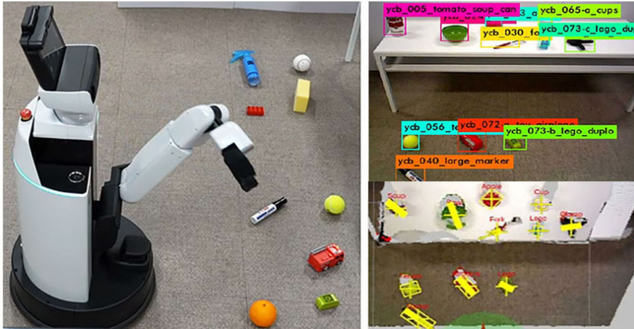
[Fig. 2] YOLO based 3D Object Recognition using Toyota HSR Home Service Robot
