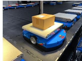
[Fig. 8] Box Sorting AGVs
