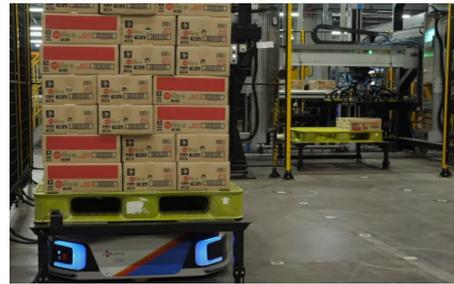
[Fig. 13] De-palletizing robot with AGV buffer system
