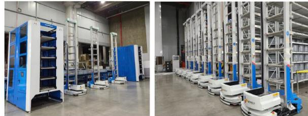
[Fig. 7] Shuttling AGVs and high rack system installed in large scale fulfillment center
