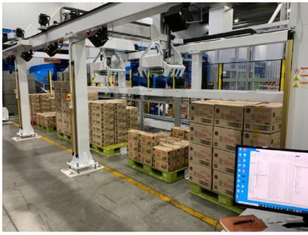
[Fig. 15] Palletizing robots supporting multiple destinations
