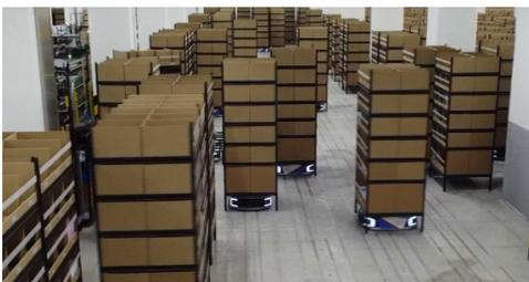
[Fig. 5] Pod transporting AGVs in fulfillment center
