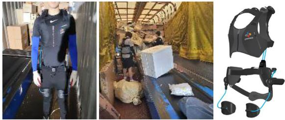
[Fig. 19] Robotic wearable device for parcel loading and un-loading<sup>[14]</sup>
