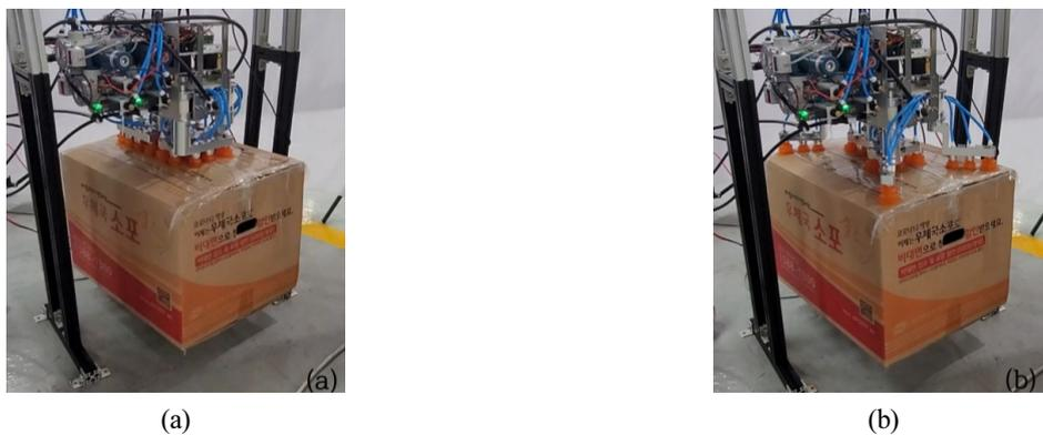
[Fig. 10] Box gripping stability experiment with adjusting working area of the gripper. (a) Gripper operation mode 4. (b) Gripper operation mode 6
