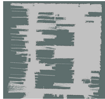
[Fig. 5] Map building result of a warehouse
