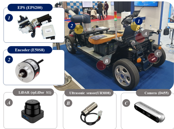
[Fig. 2] Various sensor system for autonomous driving electric vehicle
