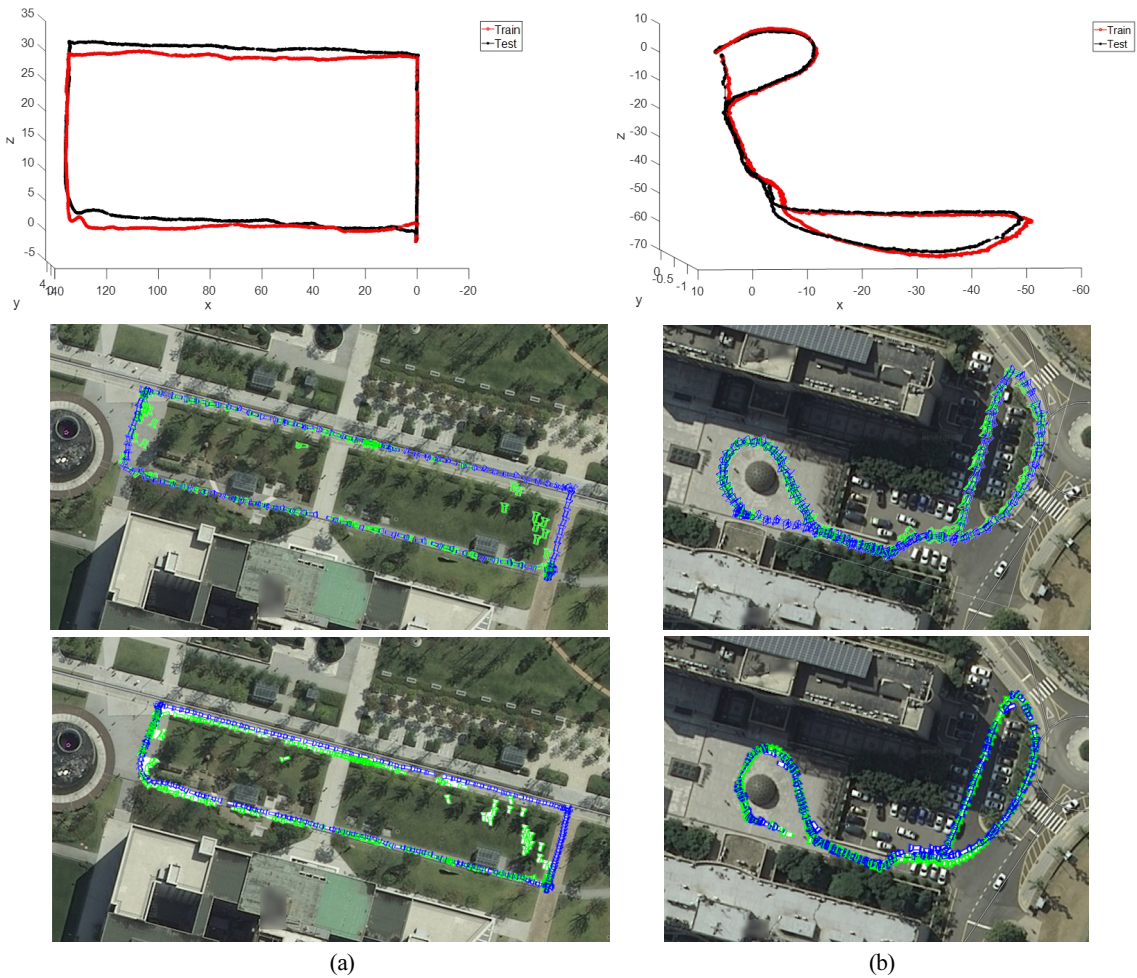
[Fig. 5] Relocalization results using our proposed method. The first row shows trajectory of training (red dot) and test (black asterisk) datasets. The second and third row show trajectory of PoseNet (green) and proposed method (blue) of Test 1 and Test2 respectively. (a) Baekyang dataset, (b) Engineering Building dataset
