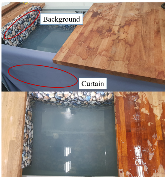
[Fig. 11] Experiment Setup. The curtain is installed to block the light from the outside. The gravel background is built in the water tank.
