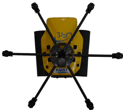
[Fig. 2] Waterproof type drone HexH2O. It is manufactured by QuadH2O company and uses handmade frame. The maximum speed is 56 km/h
