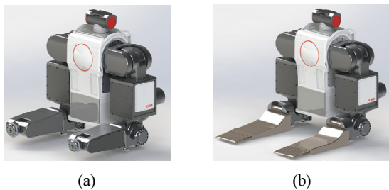
[Fig. 9] Design of dual arm robot; (a) object grasping and handling, and (b) human lifting for rescue
