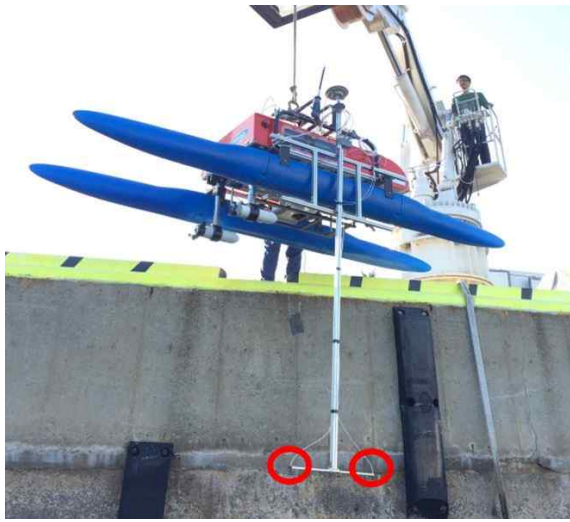
Fig. 5. Autonomous surface vehicle equipped with two hydrophones (red circles)
