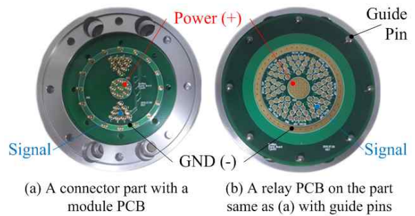
Fig. 8. Connector mechanism with communication and power bus for electrical connection
