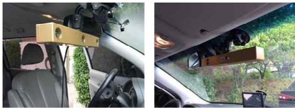
Fig. 11. Stereo vision camera mounted on the front window of a vehicle
