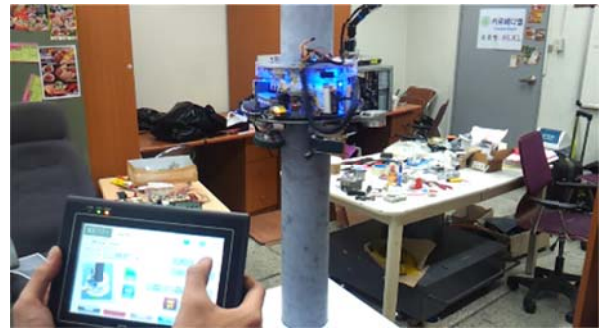
Fig. 12. Experimentation for robot ascending and descending on a column using OP panel
