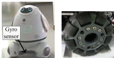
Fig. 5. Omni-wheel platform and its wheel.
