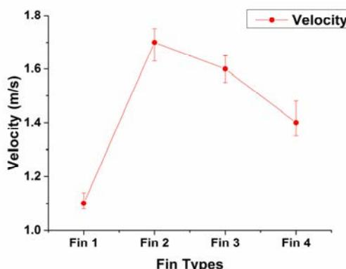
Fig. 7. Experimental results: Velocity of robotic dolphin<sup>[15]</sup>.
