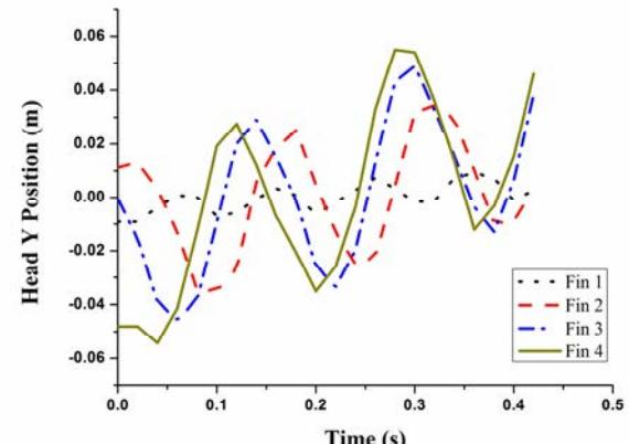
Fig. 9. Head Y position with varying the stiffness of the caudal fins<sup>[14]</sup>.
