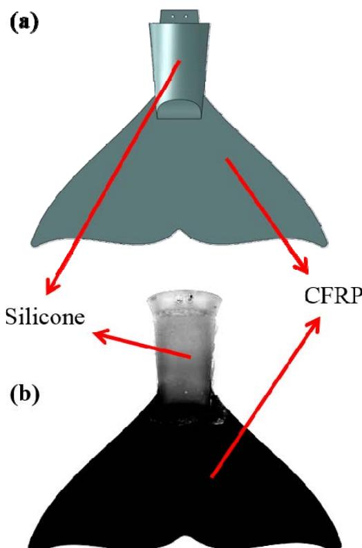
Fig. 2. (a) CAD design of a fluke, (b) Fluke which is made by CFRP laminate<sup>[15]</sup>
