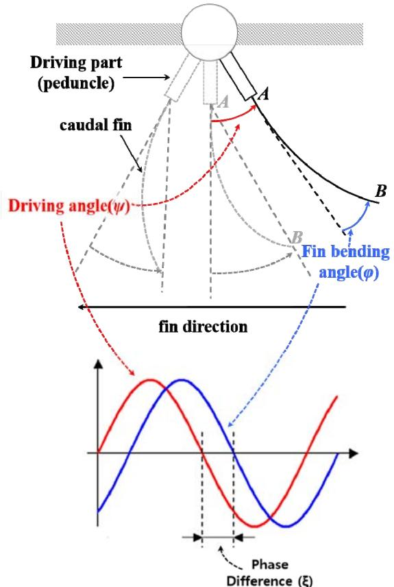
Fig. 5. The concept of the Phase difference between a driving angle and a fin-bending angle. (modified from [13])
