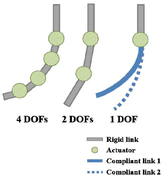
Fig. 1. Caudal fin with joints and rigid links and caudal fin with various stiffness materials<sup>[14]</sup>.
