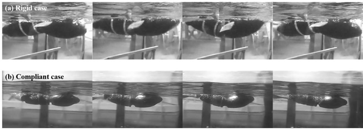
Fig. 4. Swimming motion of the robotic dolphin (a) rigid caudal fin case, (b) compliant caudal fin case<sup>[11]</sup>.
