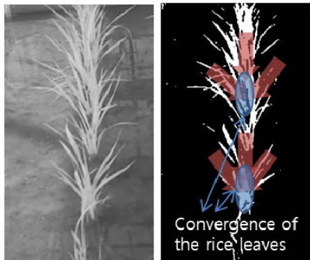
[Grey image] [Binary image] Fig. 3. Rice row perception from NIR image
