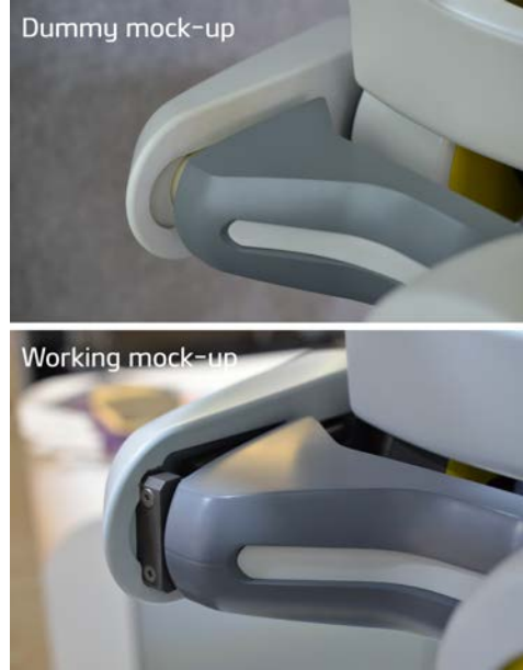
Fig. 38. Comparison between robot waist joints of dummy mock-up and working mock-up
