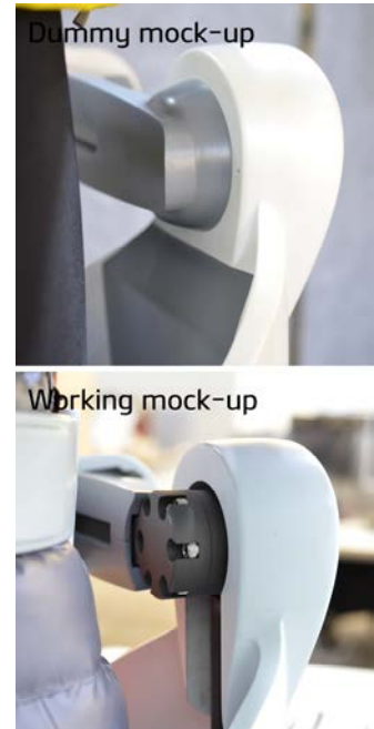
Fig. 39. Comparison between robot waist joints of dummy mock-up and working mock-up
