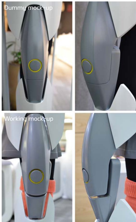
Fig. 40. Comparison between robot knee joints of dummy mock-up and working mock-up
