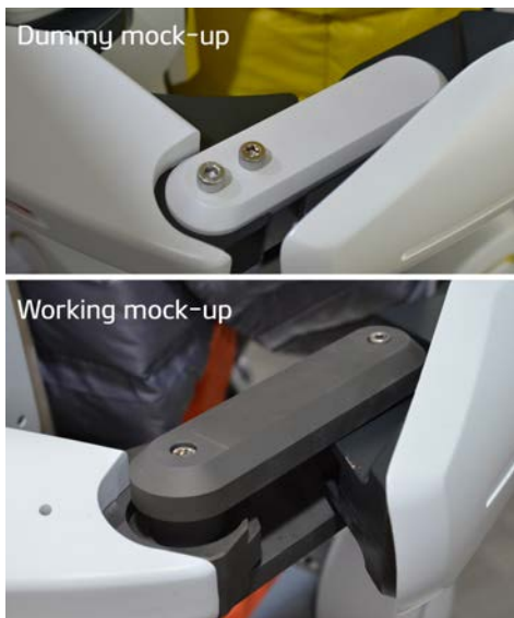
Fig. 37. Comparison between robot arm joints of dummy mock-up and working mock-up
