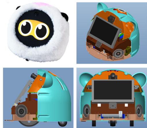
[Fig. 2] EDIE hardware CAD model and physical hardware
