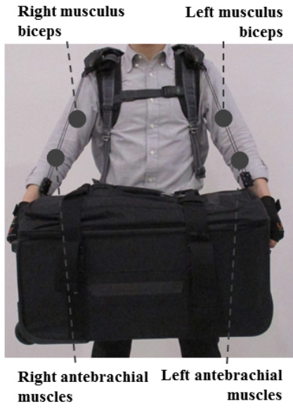
[Fig. 5] EMG sensor attachment position
