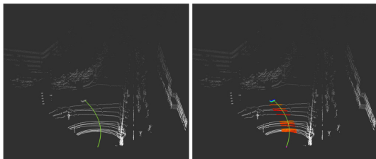
[Fig. 18] Example of point cloud ROI based waypoints
