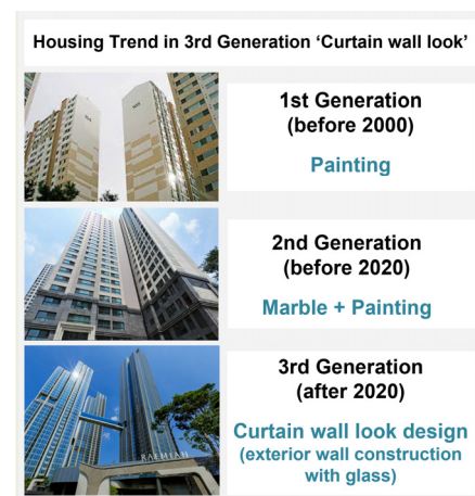
[Fig. 1] Domestic house construction trends by era: Summary about the construction trend of first-generation paint painting, second-generation marble, and third-generation curtain wall look construction
