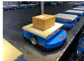
[Fig. 8] Box Sorting AGVs
