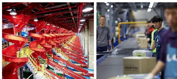
[Fig. 3] Spiral chutes and conveyors in parcel hub terminal
