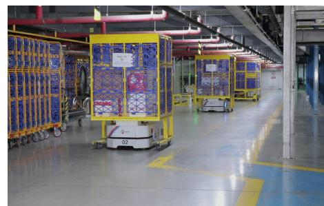
[Fig. 10] AMRs in parcel terminal for long range transporing
