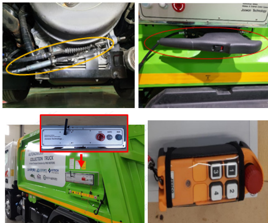
[Fig. 7] Long- and short-distance remote emergency system
