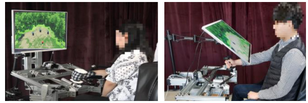
[Fig. 7] Positioning of NREH display: frontal view vs. tilted upwards from the horizontal plane [10]
