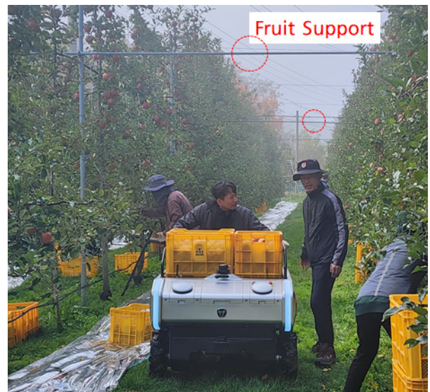
[Fig. 10] Situation of interference of RTK-GPS signals because of fruit support
