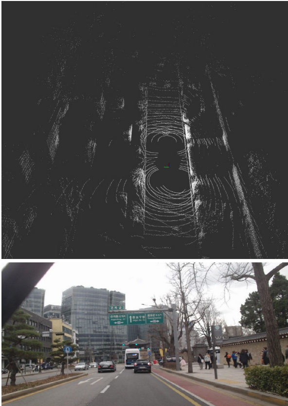
[Fig. 1] Pointcloud (up) and image (down) in the urban environment
