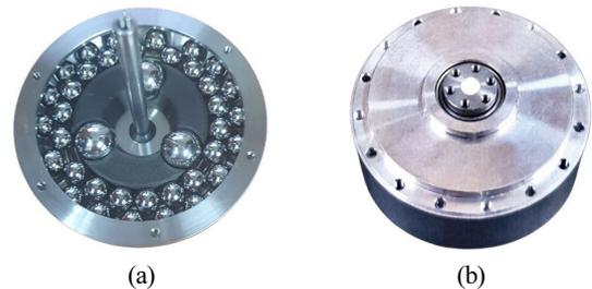
[Fig. 8] Reducer assembly process: (a) ball arrangement by jig, and (b) assembled reducer
