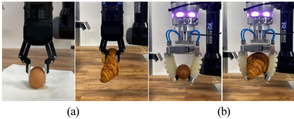
[Fig. 15] Experiments on grasping fragile and deformable objects. (a) with 2-finger gripper (broken, deformed), (b) with proposed gripper (not deformed)
