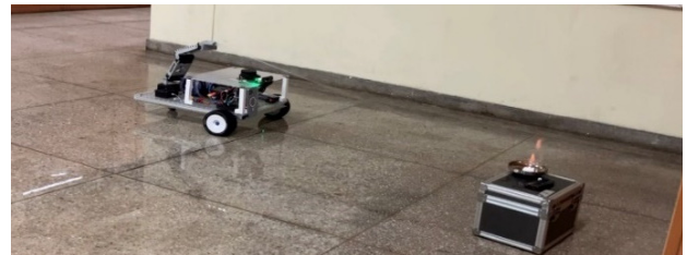
[Fig. 11] The robot (ADEFS) is extinguishing the fire
