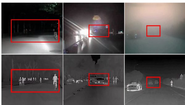
[Fig. 1] Top : RGB image, Bottom : Thermal image [7] : Within the box, the RGB image cannot accurately detect objects due to obstructions like lighting or fog, while the thermal image robustly detects objects in the same environment
