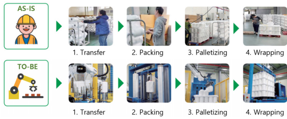
[Fig. 27] Comparison before and after robot application (bobbin transfer/loading process)
