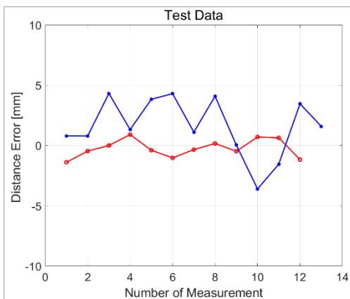
(a) Distance error before (Blue) and after (Red) calibration in training data
