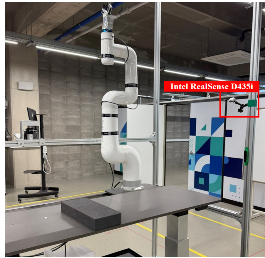
[Fig. 1] Experimental workcell configuration for object recognition: Intel RealSense D435i camera installation with workspace coverage optimization
