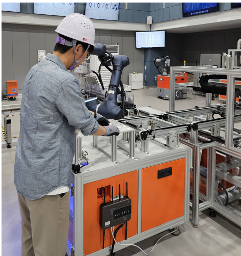
[Fig. 6] Packaging process for pet care robots with human-robot collaboration
