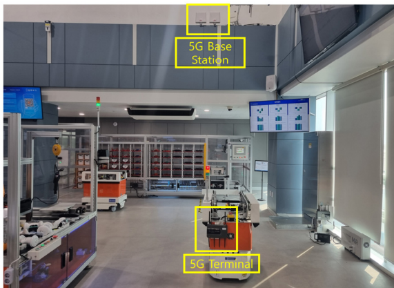
[Fig. 2] Transportation process of autonomous mobile robot within the test bed
