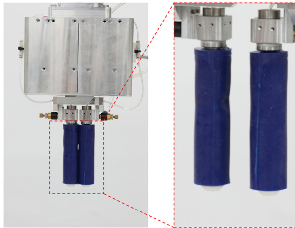
[Fig. 8] Shape adaptation and retention of the variable stiffness mechanism demonstrated by maintaining wire bundle form after removal
