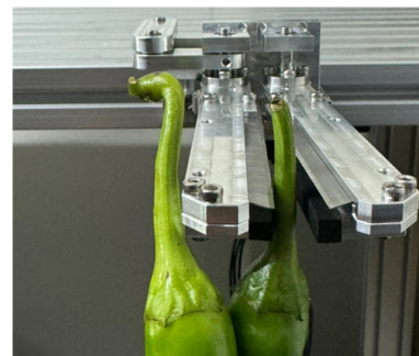
[Fig. 7] The gripper finger insertion between close pepper stems
